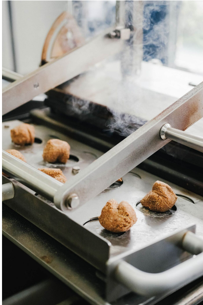
Good-Edi custom made machinery used for pressing and baking the dough balls into edible cups. Photographer: Sarah Pannell for Bloomberg Businessweek
