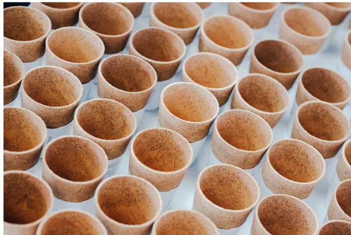
Good-Edi cups, formed and trimmed, ready to be packed in paper sleeves at the Good-Edi processing plant in Melbourne, Australia. Photographer: Sarah Pannell for Bloomberg Businessweek
